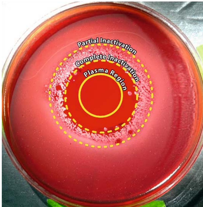
Fig. 17 Petri dish with blood agar, seeded by \sim 1.3 \times 10^7 cfu/cm 2 ( 10^9 cfu/ml) of skin flora and then treated by FE-DBD plasma for 10 s. While the plasma region diameter is roughly 25 mm, the “inner” circle of inactivated bacteria and fungi diameter is \sim 35 mm and the “outer” circle where the bacteria is partially inactivated (colonies are visible) is \sim 54 mm
